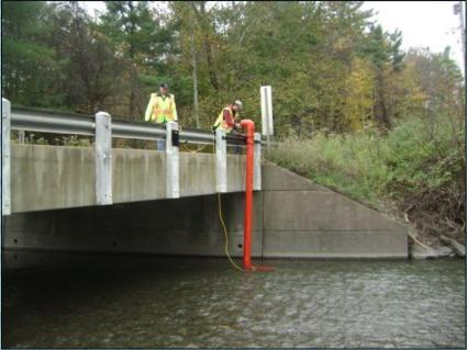
The standpipe system is easily lowered into the water and can be retrieved with minimal effort.
