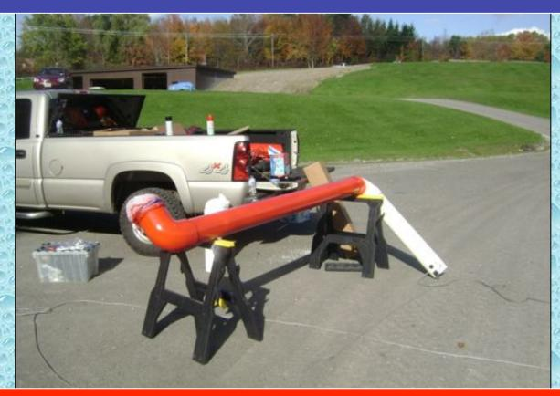
The installation used a 6-inch barrel strainer with a backflush feature that allows the pipe to be cleared of debris and sediment before drafting commences.
