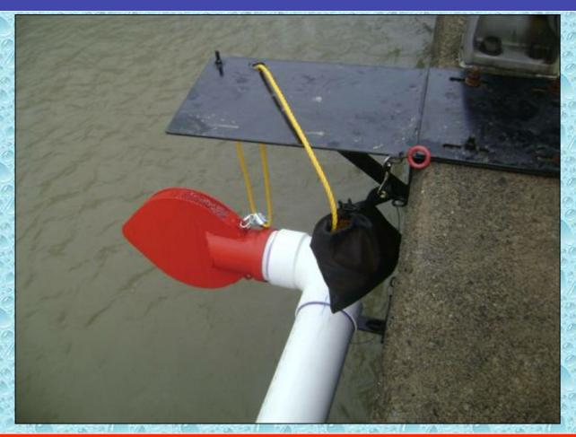
The rope bag is stored with the arm over the side of the bridge ready for use.
