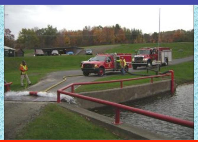
A flow of 1,000 gpm+ was obtained during the flow test. The saddle mount installation bracket allows flexibility in installation location.
