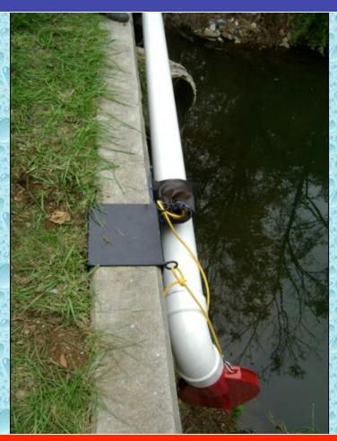
The installation required no drilling of holes and was very similar to a jersey wall, saddle mount installation.
