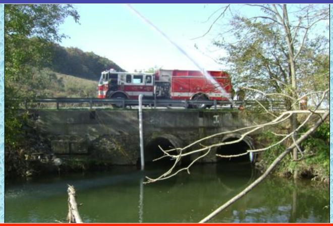
This saddle mount installation mounted to the bridge abutment wall and was equipped with a teardrop style strainer.
